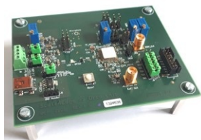
Figure 2: Demo board for keyword spotting with the test chip by TU Dresden (white, center)
