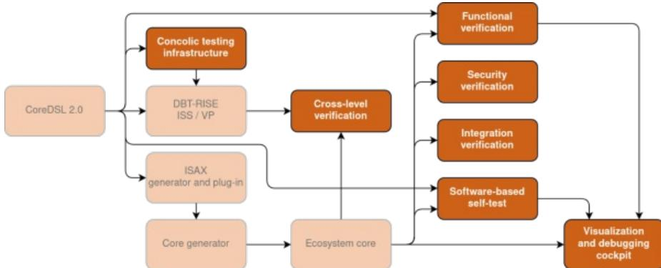
Figure 1: The Scale4Edge Hardware Verification Ecosystem
